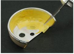
8 Another option is to cover different areas with masking tape, cut to size with a sharp-pointed cutter.
